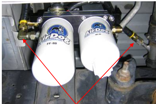
Figure 8: Connect return fuel line here
