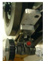
(PIC 3)Once the drive hub has been installed, move on to the base plate, this installs by removing the front 4 bolts on the pan rail, then install the 4 supplied bolts. Then move to the next step.
